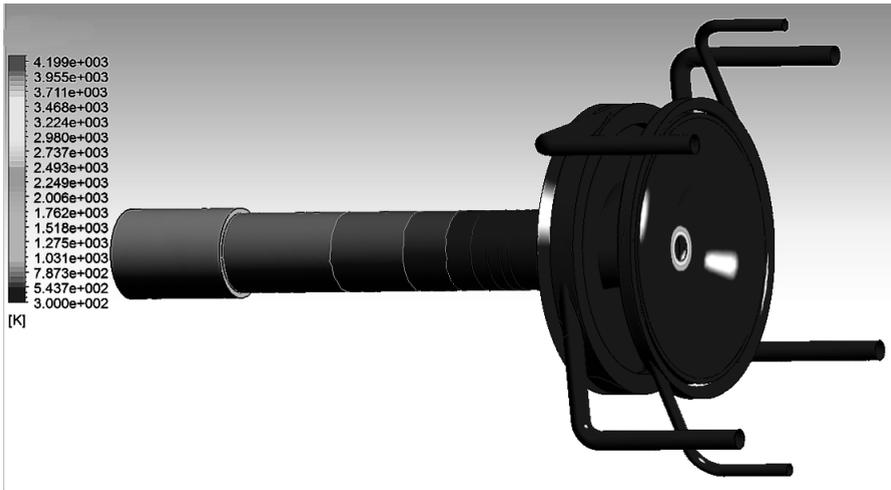
Figure 6 – Temperature distribution on the wall of the plasma torch channel [4]
