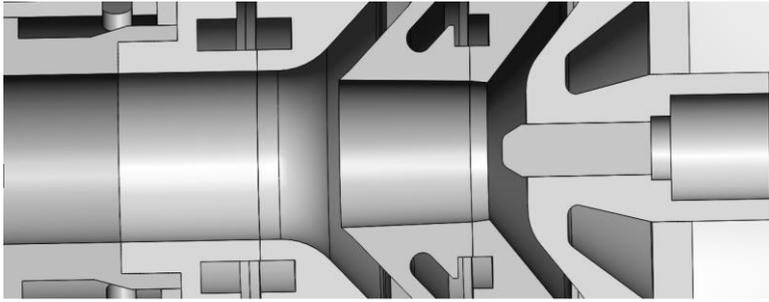
Figure 4 – Modified geometry of the plasmatron flowing part [5]
