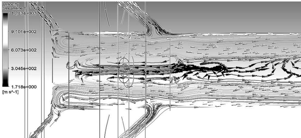
Figure 3 – Velocity distribution in the cathode space[4]
