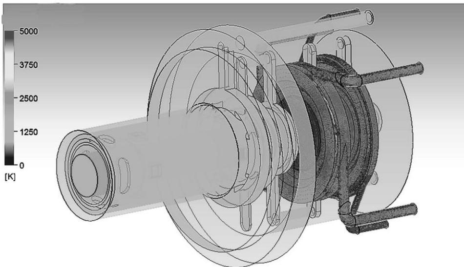
Figure 7 – Temperature distribution on the wall of the plasma torch housing[8.9]
