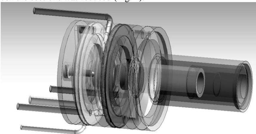
Figure 1 – Geometry of the modernized plasmatron[3,4 ]
