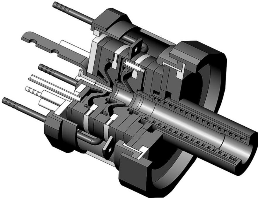
Figure 11 - Three-dimensional model of the developed plasmatron[4.10]
