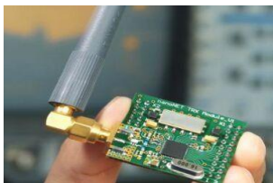
Figure 2. Active RFID tag with a changeable antenna[6]
